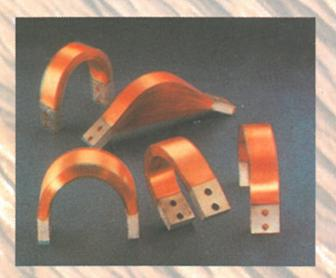
For a long time the concept of copper flexible was just stacking together bunches of foils and connecting the same. Further, rivetting at the ends was started and was further improved by soldering/brazing. But the loss of energy was never considered/assessed. Later on, as the cost of energy increased tremendously, the technique of hot pressure fusion welding process was put in use which is the latest trend and resulting into substantial savings in energy cost. SRG is using the same technique.
